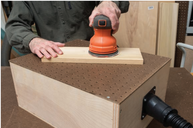
A downdraft sanding box directs air through a pegboard top into a shop vacuum and keeps airborne dust from sanding under control.
