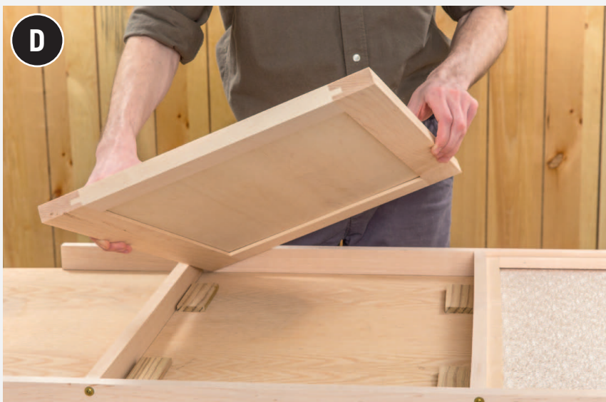
With even spacing, set a door panel into each bottom frame opening. Attach the doors by driving brads through the uprights and the bottom rail.
