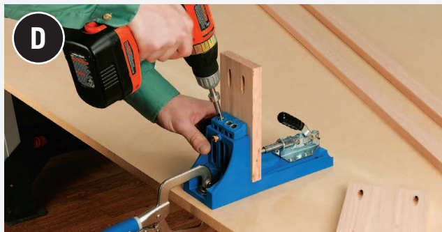
Use a pocket-hole jig as a guide to drill the pocket screw guide holes.
