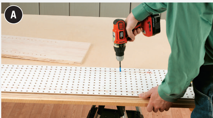
Use perforated hardboard as a guide to drilling the shelf-pin holes.
