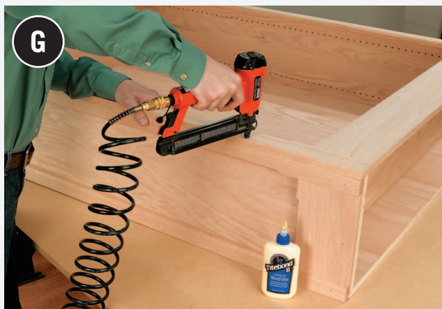
Attach the front and back face frames to the cabinet.
