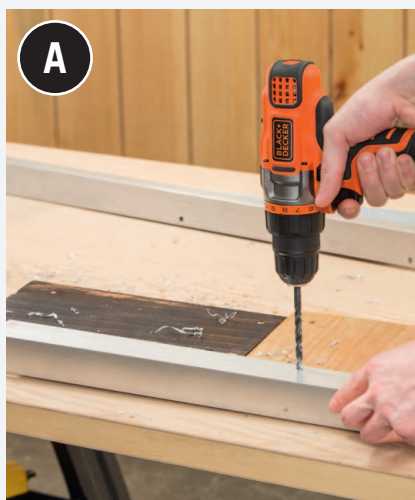
Drill guide holes in the aluminum angle legs for the screws that will attach the shelves.
