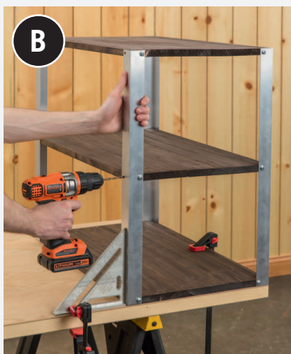
Attach the finished shelves to the legs.
