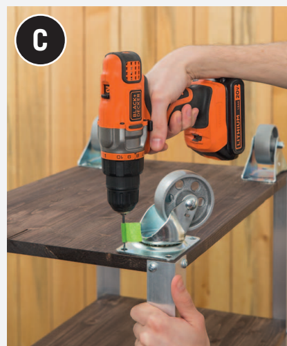
Attach the fixed casters on one end and the pivoting casters on the other.
