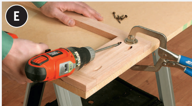
Assemble the face frames with glue and pocket screws.
