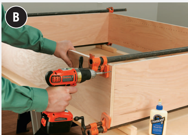
Assemble the carcase with glue and screws.
