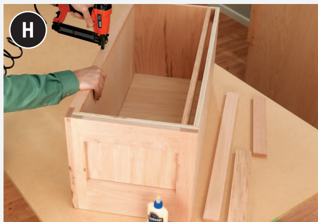
Attach the bench caps to the top of the bench assembly.
