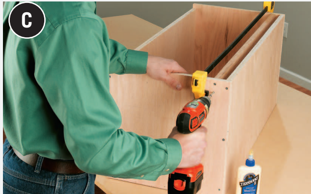
Attach the lid rail between the carcass sides.
