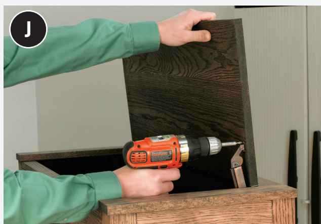
Install the lid hinges and support hardware.
