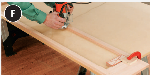
Make chamfer cuts on the face frame with a router.
