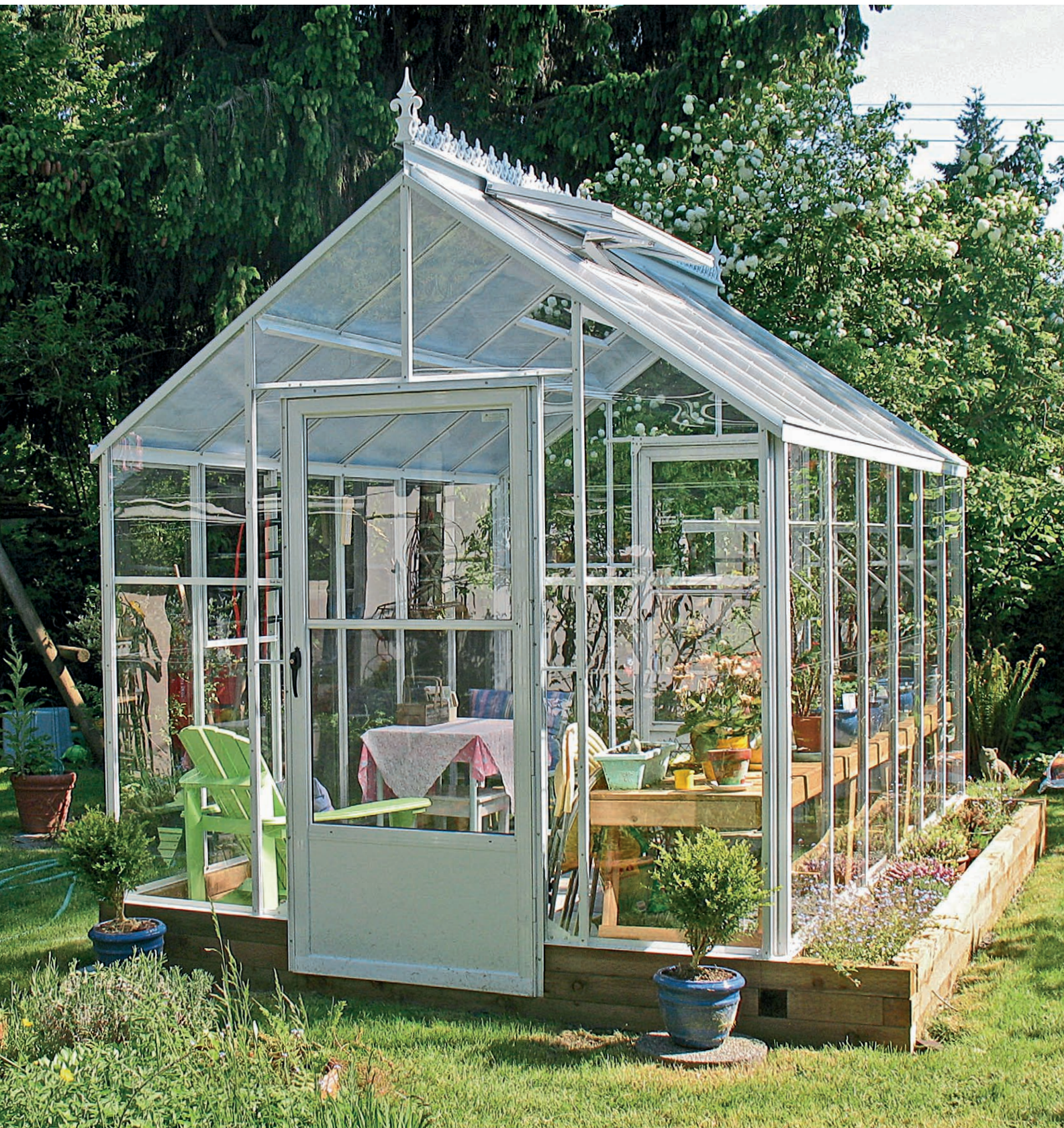
This large Victorian-style glass greenhouse features a “drop” door—a door that extends down below the original threshold of the greenhouse to accommodate the height of a foundation wall. The steep roof pitch and distinctive top crest create an eye-catching formal visual with plenty of space inside for growing a variety of plants or just relaxing in the warmth of the sun.
