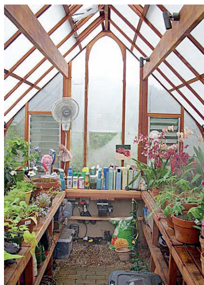
A pine frame with plastic glazing. This is a good option for a lightweight and inexpensive greenhouse that will be used for two or three seasons.
