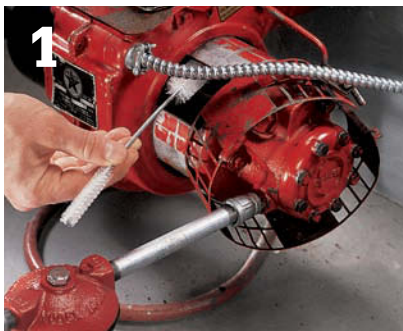
To clean the air intake , use a brush designed for cleaning the condensing coils on a refrigerator.
