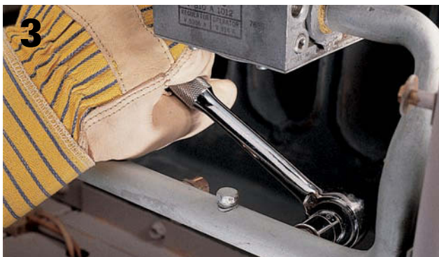
To avoid bending or damaging the spud threads, hold the manifold steady with one hand as you remove each spud.
