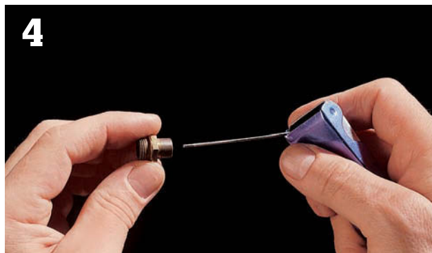
Clean each spud orifice carefully with a pilot jet tool, taking care not to scratch or enlarge the orifice.
