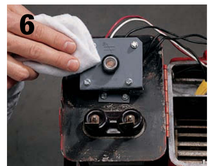
If the motor doesn't have cups or openings for adding lubricating oil, it's probably sealed and may not need extra lubrication.
