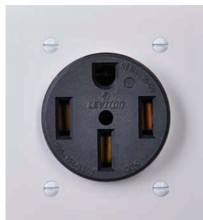
50 amps, 120/240 volts. This new, grounded receptacle is used for ranges. The high voltage powers heating coils, and the 120-volts run clocks and lights.
