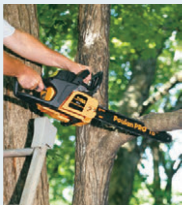
Start by undercutting from beneath the limb with your bow saw or chain saw.
