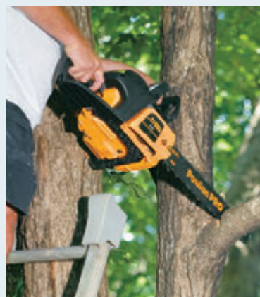
Trim the stub from the limb so it's flush with the branch collar.
