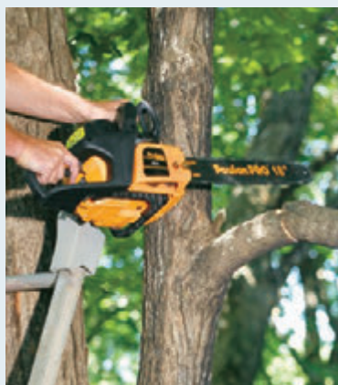
Finish the cut from above —this keeps the bark from tearing when the limb breaks loose.
