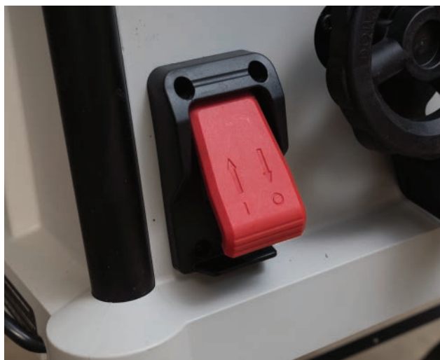
Another important tablesaw safety feature is a paddle switch that must be pulled out to start the tool, and can be turned off by pressing it with your knee.
