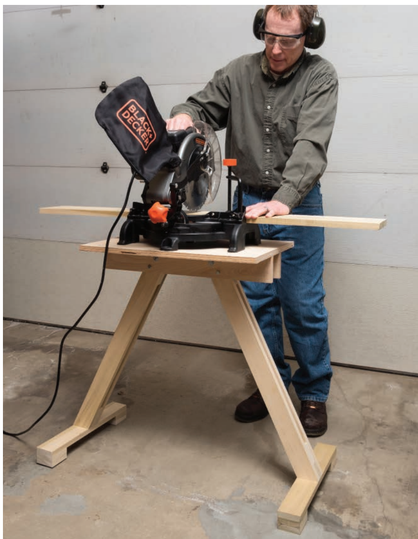
This folding miter saw stand is lightweight, is easy to transport, and can support any small- to medium-size saw. It can also double as a shop utility table. Fasten the miter saw to the stand with at least two bolts and wing nuts to keep it secured while working.
