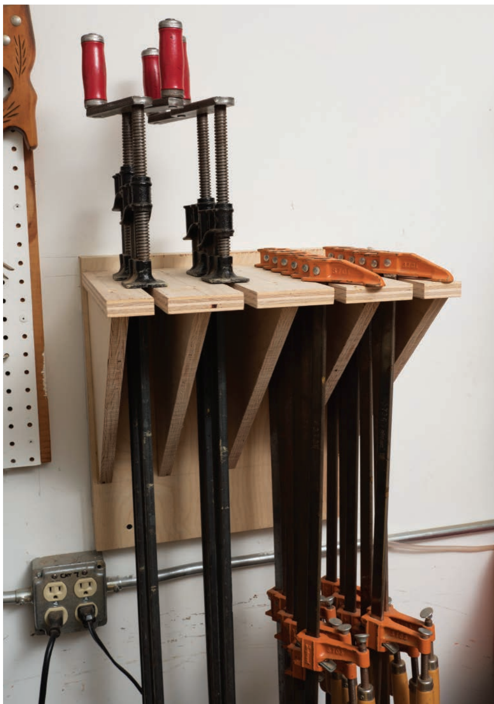
The capacity and type of clamps this rack accommodates can be easily modified by making it wider and changing the width of its slots.
