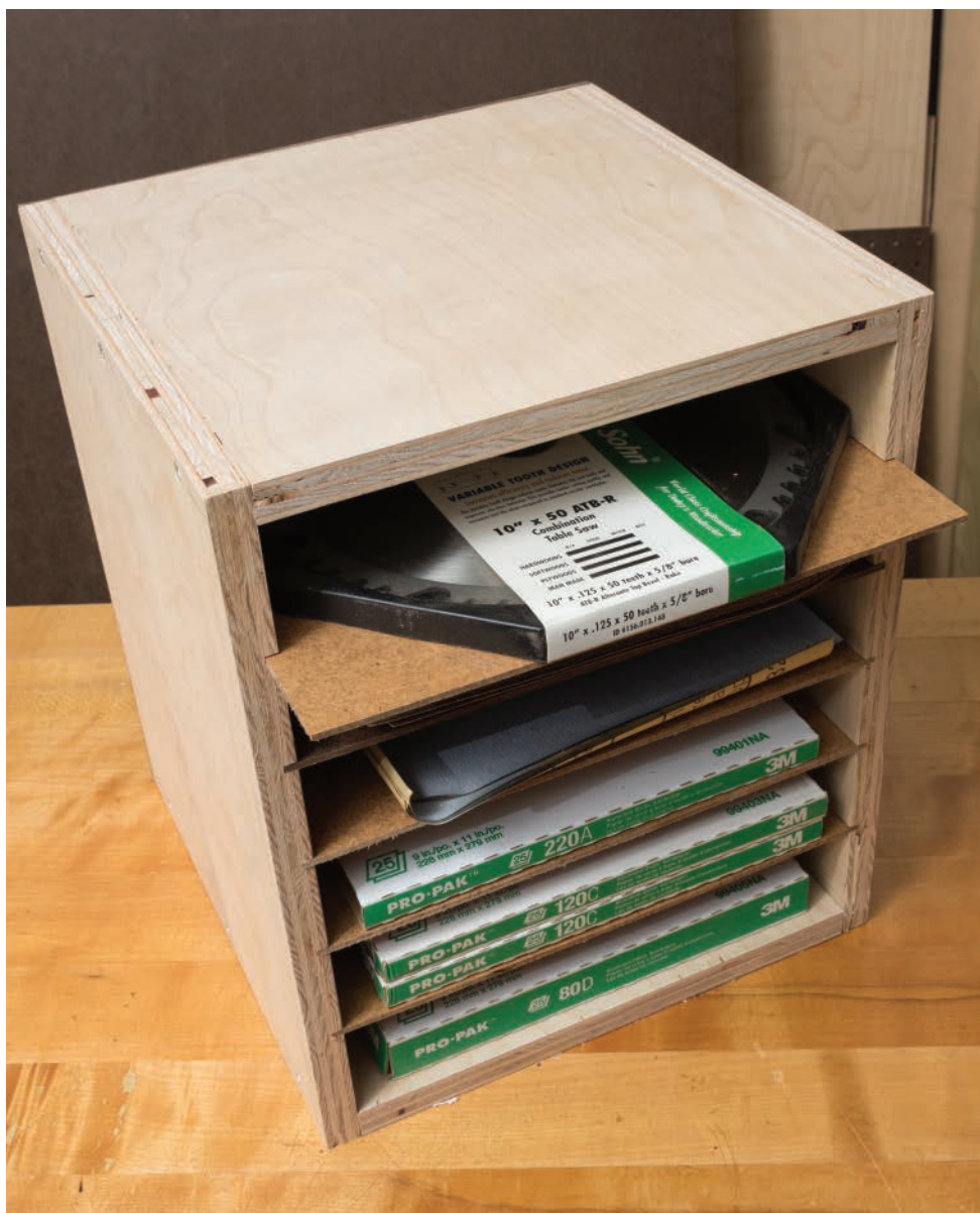
A sandpaper storage box is also practical for keeping saw blades organized. Simple construction and sliding shelves make this a quick and versatile project.
