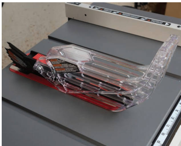
All currently produced tablesaws have a blade guard, a riving knife, and anti-kickback pawls that should be used whenever making through cuts.
