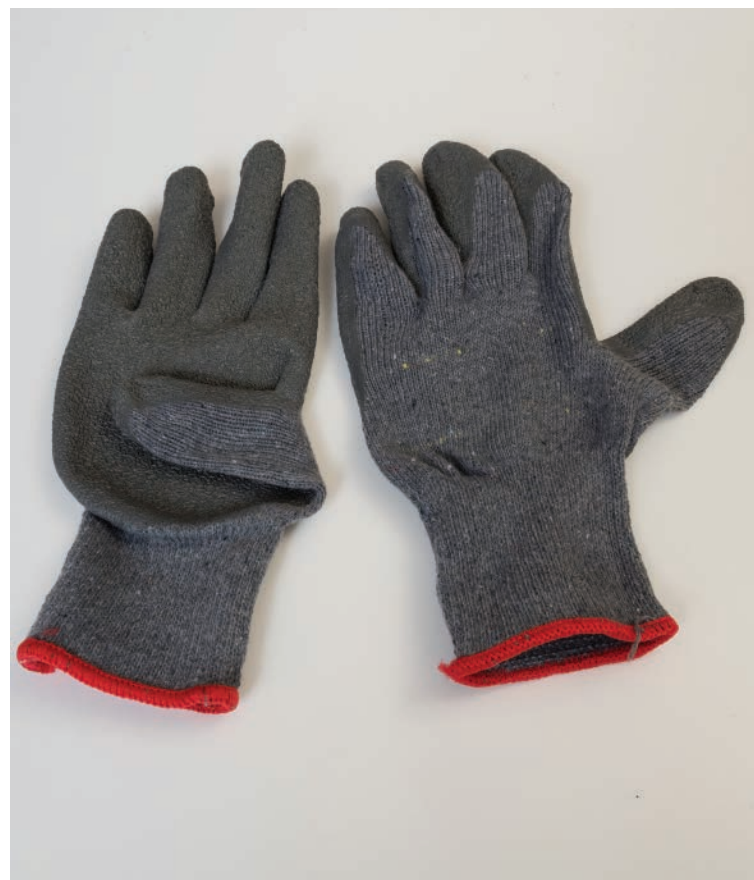
Knit rubber-coated gloves are relatively cool to wear and they're useful for many shop applications, including finishing.
