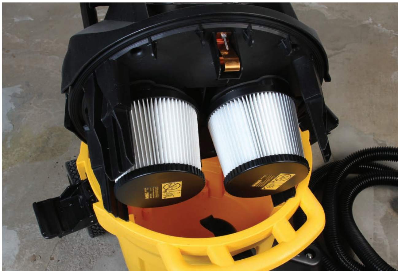
HEPA filters on dust extractors remove even the finest dust produced by tools. Most standard shop vacuums don't provide this level of filtration.
