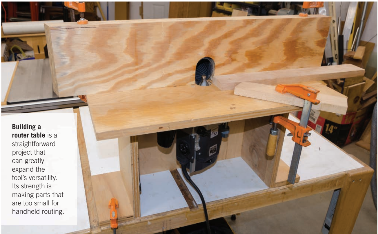
A handheld plunge router is an extremely versatile woodworking tool that can make internal cuts, form edges, and reproduce workpieces precisely using templates.
