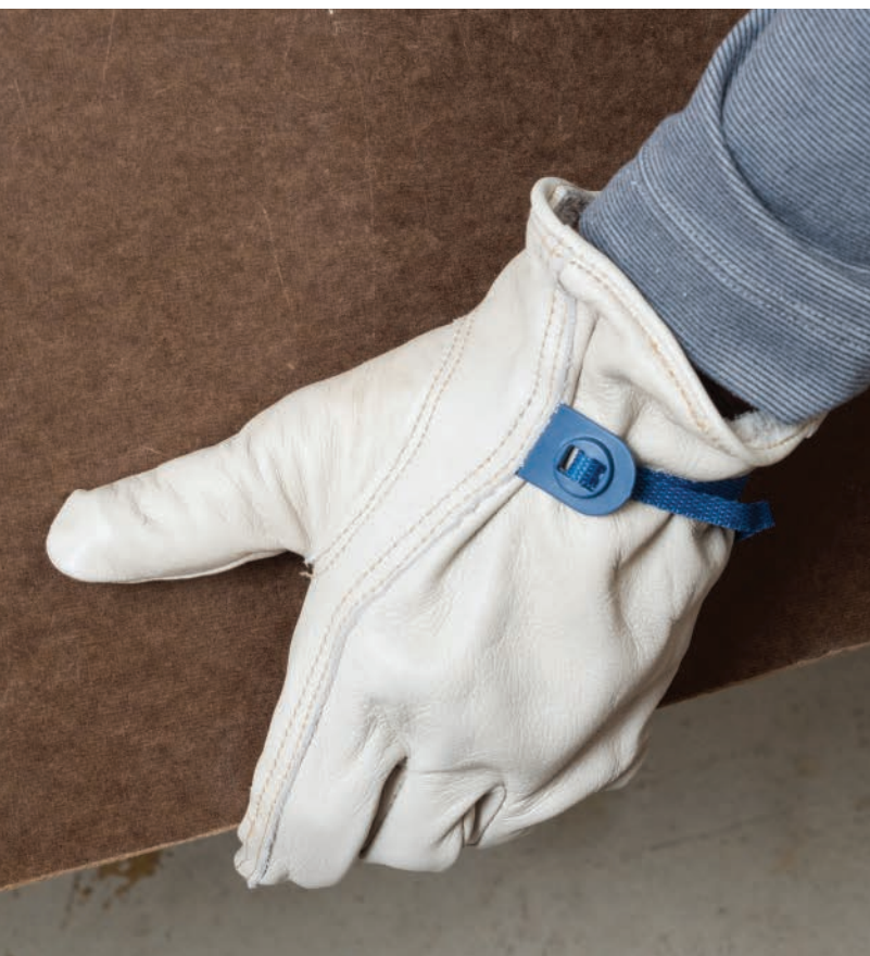
Leather work gloves provide excellent protection for carrying lumber products because they're virtually splinter proof.
