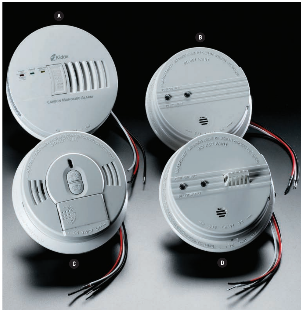
Shops are susceptible to fires , so a smoke/CO detector is essential and may be required by code in some communities. Models shown here include: (A) hard-wired CO detector; (B) ionizing smoke detector; (C) photoelectric smoke detector; (D) heat-activated fire detector.
