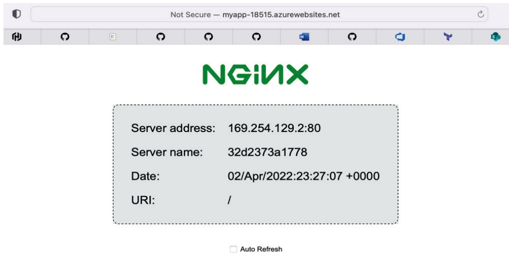
Figure 13.2 – NGINX running in Azure App Service
