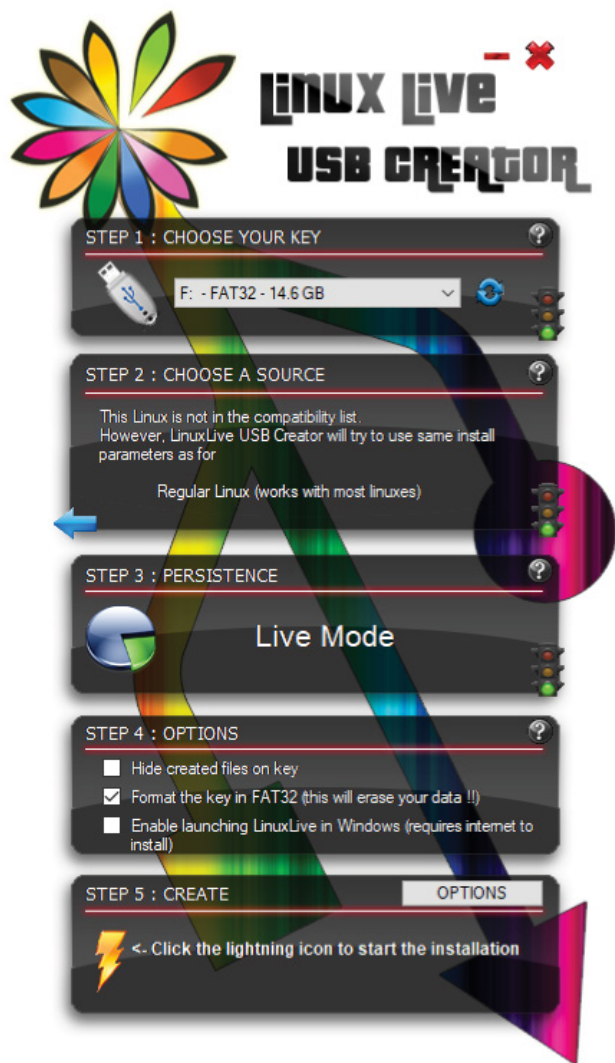
Figure 6.6: Creating a bootable Paladin USB
