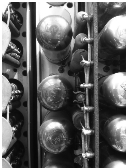
Vacuum tubes in a UNIVAC I computer Image: Diomidis Spinellis, CC BY-SA 4.0
