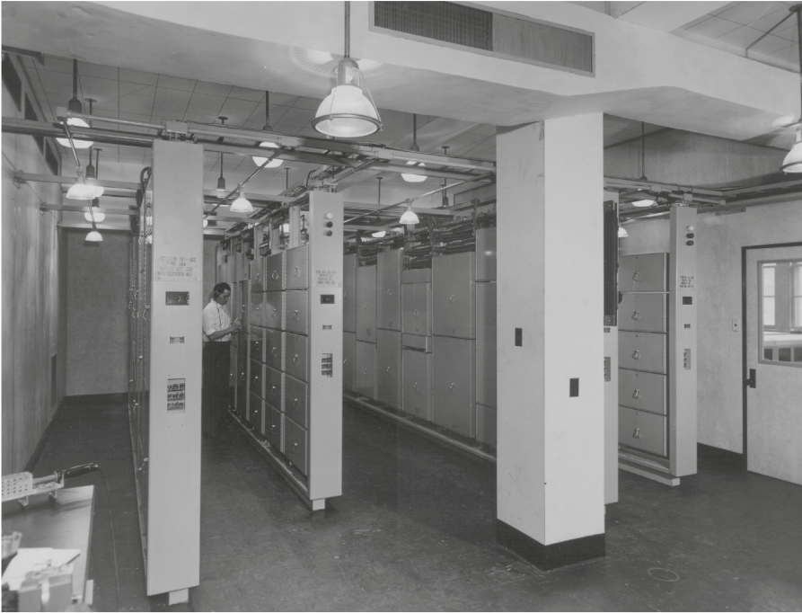
Relay equipment room of the Model V – a successor to the Complex Number Calculator – installed at Ballistics Research Laboratories, Aberdeen, Maryland US Army photo, Public Domain
