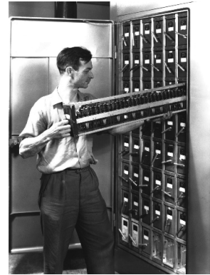
Sid Barton with the EDSAC 2 and its miniature valves Image: copyright Department of Computer Science and Technology, University of Cambridge. Reproduced by permission
